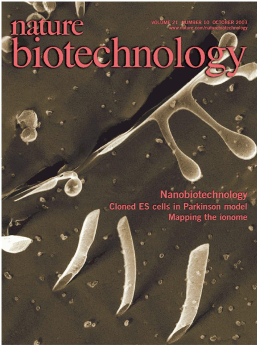
Quick-freeze深深-etch transmission electron microscope (TEM) images of a solution of peptides that form peptide nanotubes. There are also vesicles budding off of a nanotube and micelles in the area. Peptide nanotubes may provide new biomaterials for materials science and biology research (see [Zhang, p. 1171](#)). Peptide nanotubes prepared by Sylvain Vauthay and Steve Santoso. Artwork rendered by Erin Boyle.
